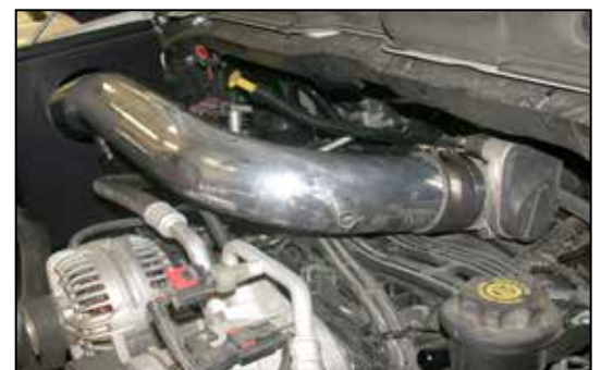
26. Slide the intake tube into the heat shield then slide the tube into the silicone hose on the throttle body as shown, but do not tighten completely at this time.
