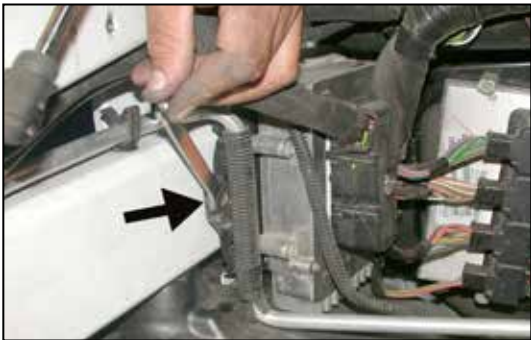
12. Remove the screw that secures the computer to the inner fender as shown.
