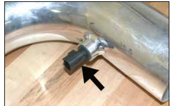
25. Slide the air temperature sensor into the silicone hose as shown. NOTE: The plastic cage on the end of the air temperature sensor is very fragile so take care when installing the air temperature sensor into the silicone hose.
