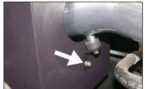
27. Secure the angle bracket to the heat shield using the provided hardware as shown, but do not tighten completely at this time.
