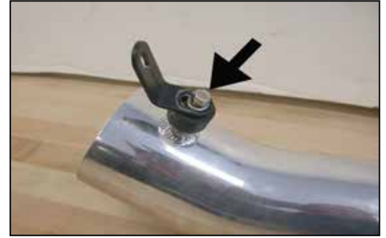
23. Install the angled bracket onto the rubber mounted stud using the provided hardware as shown, but do not tighten completely at this time.
