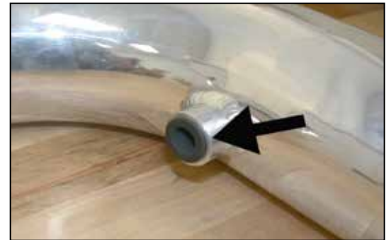
24. Install the provided silicone hose into the vent on the K&N® intake tube as shown.
